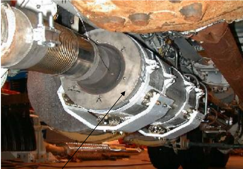
1 kW e TE Mounted under PACCAR vehicle Tested for ~500,000 equivalent miles
